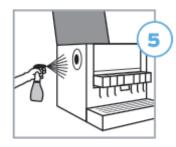
Spray exterior food contact surface area with food contact sanitizer. Ensure treated surfaces remain wet for contact time indicated on product label. Allow to air dry. Reinstall nozzles, diffusers and cup rest. Fill ice bin with fresh ice (if applicable).
