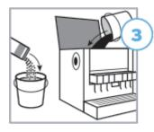
To sanitize ice bin (if present): Sanitize interior of unit with **food contact sanitizer** and allow solution to soak per time specified by product label before draining. Allow to dry. Do not rinse.
