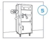
Return unit to proper temperature. Use a multi-purpose disinfectant for the exterior, ensuring proper disinfection of high-touch, non-food contact areas like handle. If needed. use **stainless steel** cleaner and a clean, soft cloth to shine exterior.
