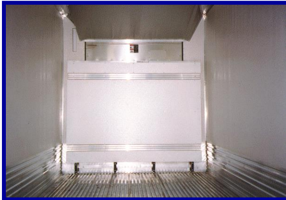
Clean trailer w/ attached air chute
